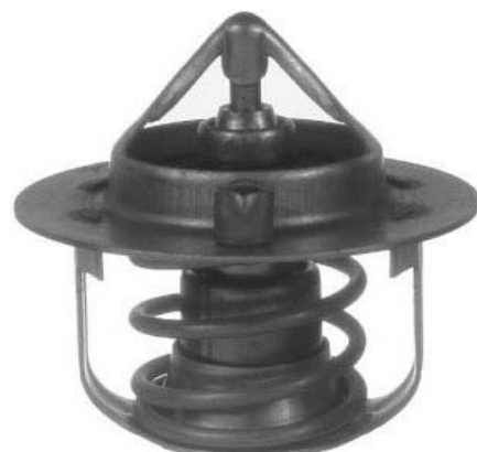
Jiggle pin inversed / Rubber valve
